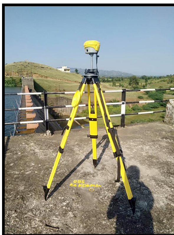
Figure 5.3-1 RTK Base Set up At Dam
