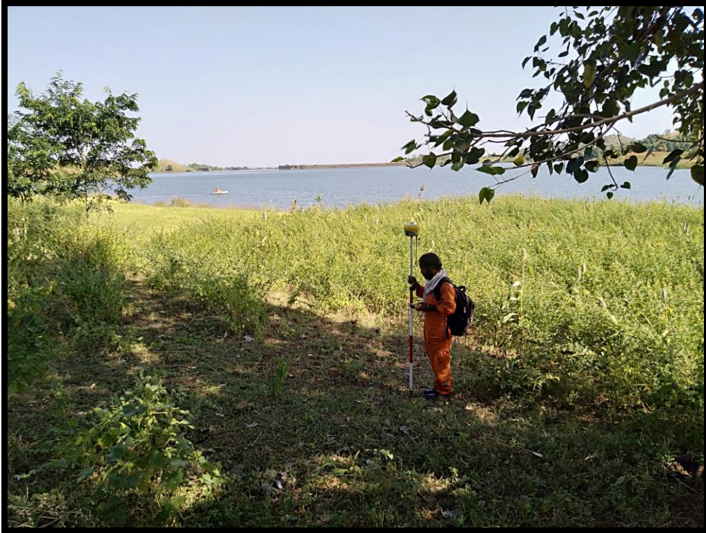
Spot fixing with RTK Rover
